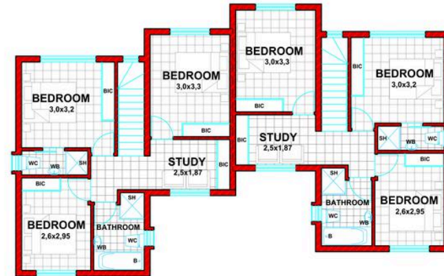
UNIT TYPE A FIRST FLOOR PLAN 1:100
